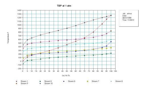
This example explains usage of the Tower Plus distillation model and the way of performing crude oil characterization.
