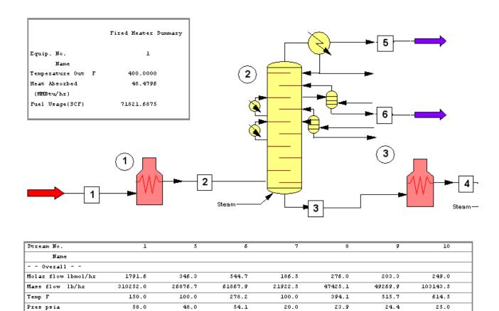
Databoxes and graphics can be placed directly on flowsheet, forming together Main Process Flow Diagram. Individual Process Flow Diagrams can be also created and edited.
