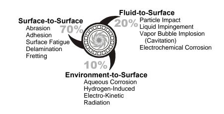
The frequency in which various wear modes occur in practice depends upon the type of equipment, the environment and the duty cycle severity. A table giving the relative frequencies of the various wear modes is presented below:
