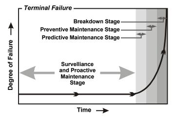
Following the incipient failure stage, a stage called impending failure eventually takes place, as expressed in Fig. 4. This stage is manifested by the degradation of system performance and prompted by the continued loss of critical surface material. Due to the damage that occurs, this is the stage where failure becomes totally irreversible.
